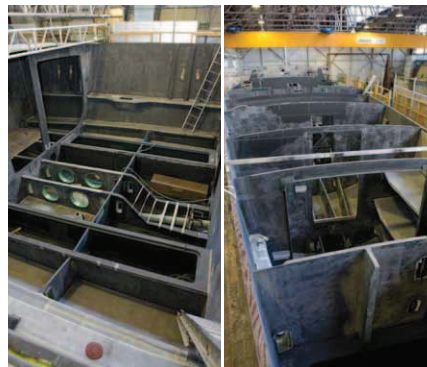
OPPOSITE: FINITE ELEMENT ANALYSIS (FEA) RENDERING OF SARISSA SAILING UPWIND BY TRIPP DESIGN, SHOWING HER INTERNAL CARBON STRUCTURE AND STRESS LEVELS. BLUE AREAS ARE HIGH STRESS, RED AREAS ARE LOW STRESS. LEFT: SARISSA UNDER CONSTRUCTION AT GREEN MARINE. A CARBON YACHT REQUIRES MORE UPFRONT ENGINEERING AND PLANNING AT THE START OF THE PROJECT SO THAT ALL THE STRUCTURAL ELEMENTS ARE INCLUDED BEFORE THE HULL IS HEAT CURED. IMAGES BY ALBERT BRUNSTING & RENDERING BY TRIPP DESIGN.
