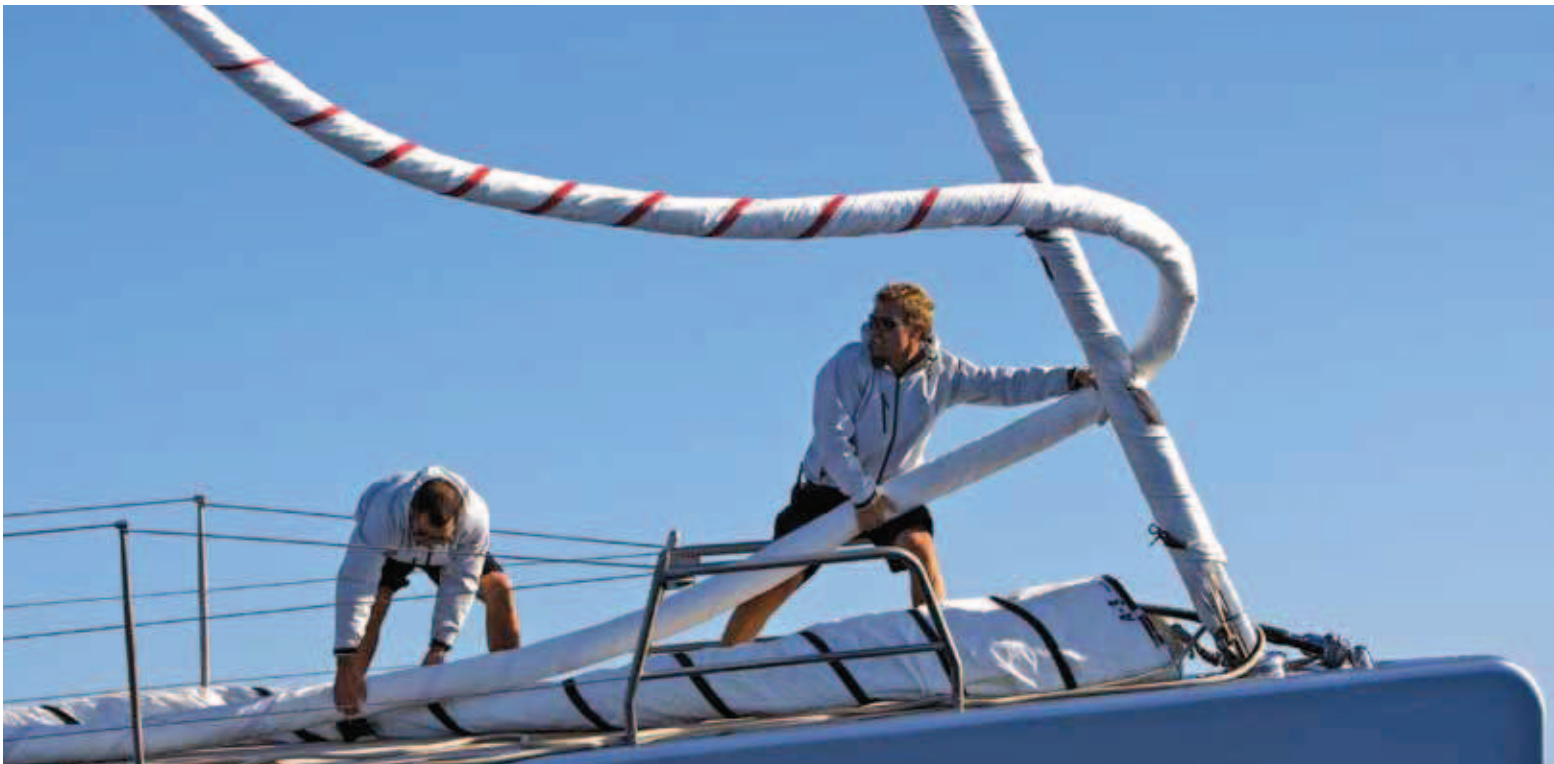
1,150SQM A3 ASYMMETRIC SETS ON A HYDRAULIC CABLE FURLER ON THE BOW.
